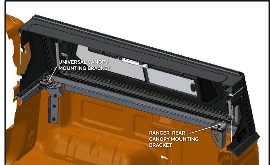
Fig 21. Position of Canopy Mounting Brackets
